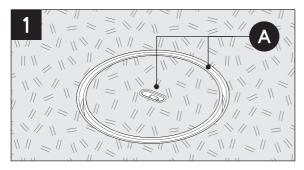
Ensure outer rim slot and central opening of Lid (A) remain free of any blockages, dirt and other debris.
