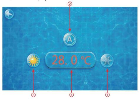
Click the refrigeration mode button ①, automatic mode button② or heating mode button ③then you can select the corresponding mode.
