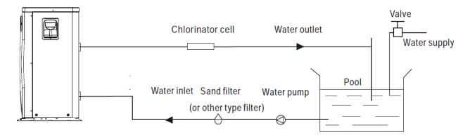
The factory only provides the main unit and the water unit, other items in the illustration above are necessary spare parts for the water system that are to be provided by the user or the installer.
