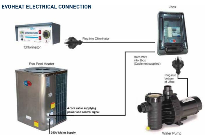
NOTE: heat pump, Jbox and water pump all on the same circuit
